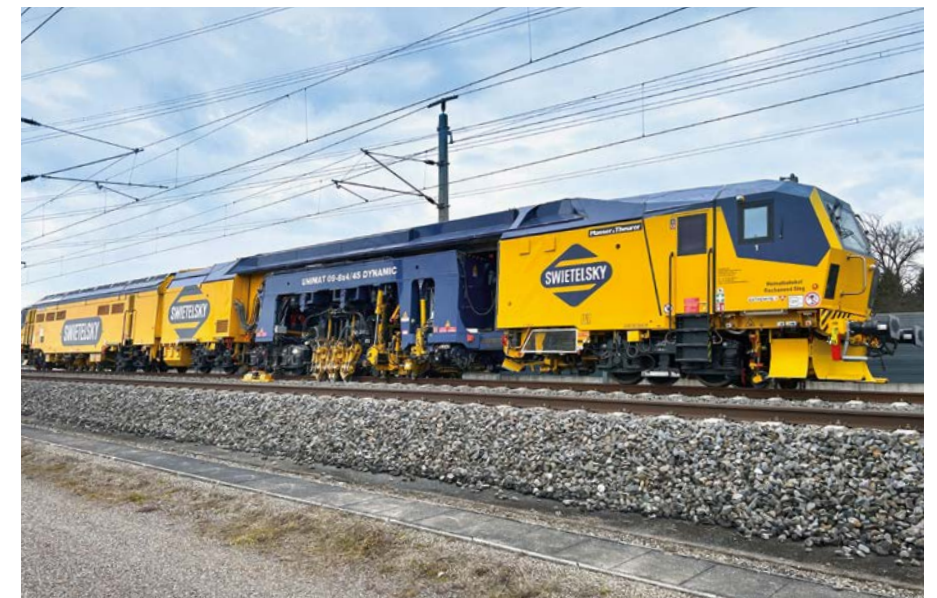
UNIMAT 09-8×4/4S Dynamic Tamping Machine
